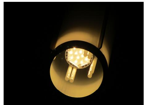
Testing was done with a prototype to ensure that the light output of the whole project would meet the church's needs. All of the lights can be easily dimmed and controlled with a wireless remote.
